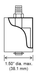
MS8000 comes with integrated slosh guard. Bottom of slosh guard takes the place of the float switch bottom clip.
