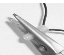
3c Add crimp caps to the twisted pairs and crimp very firmly with pliers.
