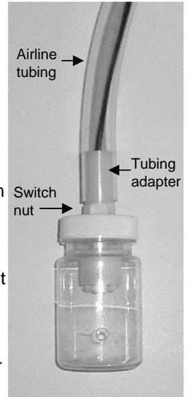
2. Wire the third float switch into the float switch assembly following Step 3 of the main instructions and adding it as shown below. Place the reservoir switch in the bottom of your reservoir. Keep the top of the tubing above the high-water level.
