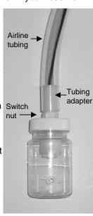
2. Wire the third float switch into the float switch assembly following Step 3 of the main instructions and adding it as shown below. Place the reservoir switch in the bottom of your reservoir. Keep the top of the tubing above the high-water level.
